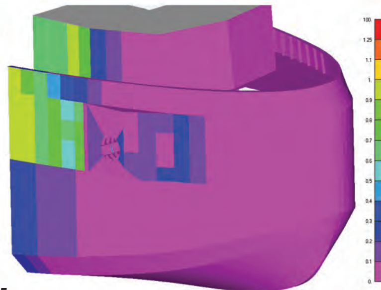
Figure 5: Color Coded Buckling Assessment Plot using ABS Rules for Multiple Load cases.
